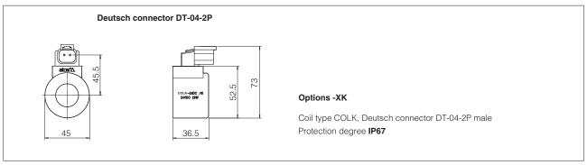
Note: For the electric characteristics refer to standard coils features - see section 6
